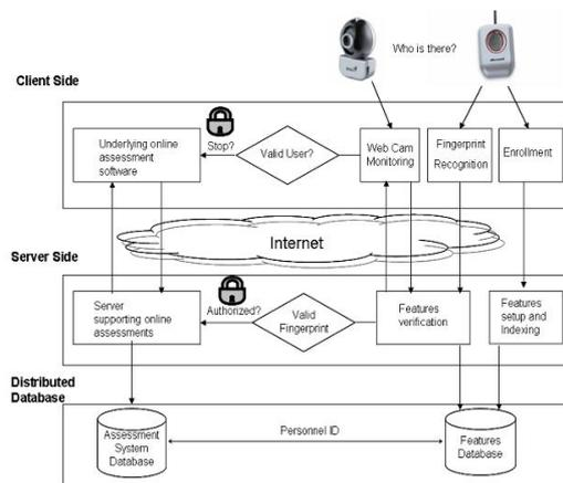
**Fig. 1.** Fingerprint recognition on real time.
